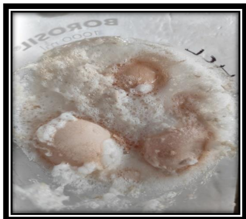
Fig. 3: Decalcification process of eggshell in 2M HCl
