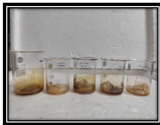
Fig. 7: Semipermeable membrane after being titrated with potassium permanganate (0.9494 N)
